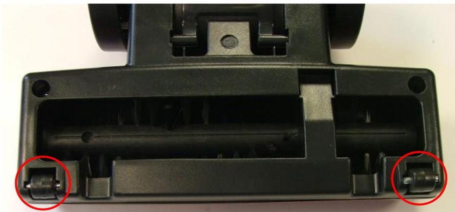
Finally prise open the flap/cover on the underside of the assembly (highlighted in yellow) and check that the drive assembly can rotate and that as it rotates the brush bar also turns.
